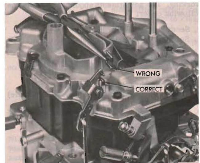
Figure 17. Correct Installation of Pump Rod "S" Link
