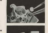
12. Remove pump jet plug and gasket assembly and pump
